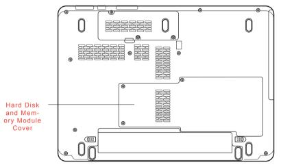
Removing the memory module cover
